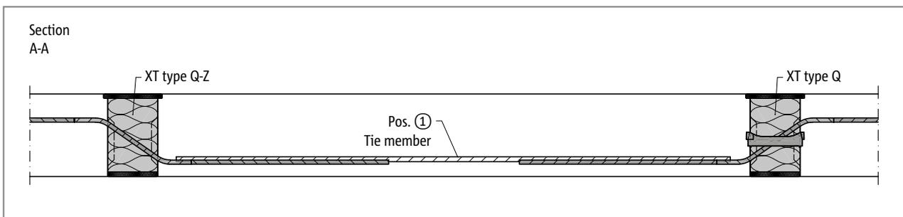
Fig. 148: Schöck Isokorb® XT type Q-Z-V5 to Q-Z-V8, Q-V5 to Q-V8: Section A-A; one direction spanned reinforced concrete slab
