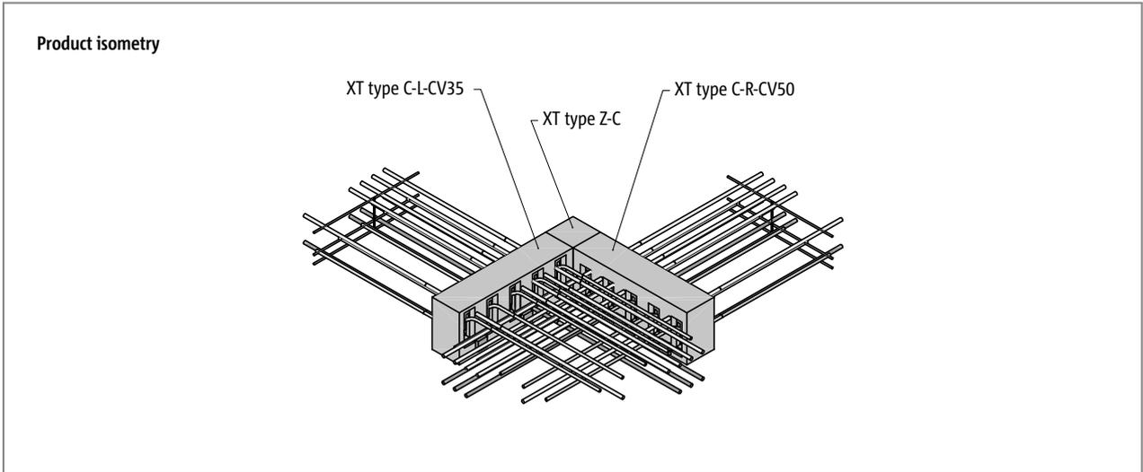
Fig. 52: change representation to illustration Schöck Isokorb® XT type C-L-CV35, XT type C-R-CV50: Isometric representation
