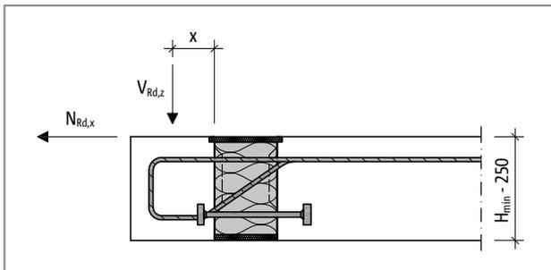
Fig. 249: Schöck Isokorb® XT type O: Distance of the load application point  $x$  (load distance point)
