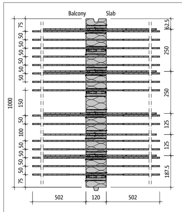
Fig. 32: Schöck Isokorb® XT type K-M6: Product plan view
