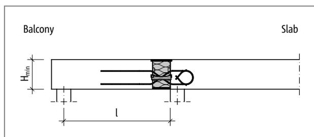
Fig. 131: Schöck Isokorb® XT type Q-VV: Static system (XT type Q-VV1 to VV4)
