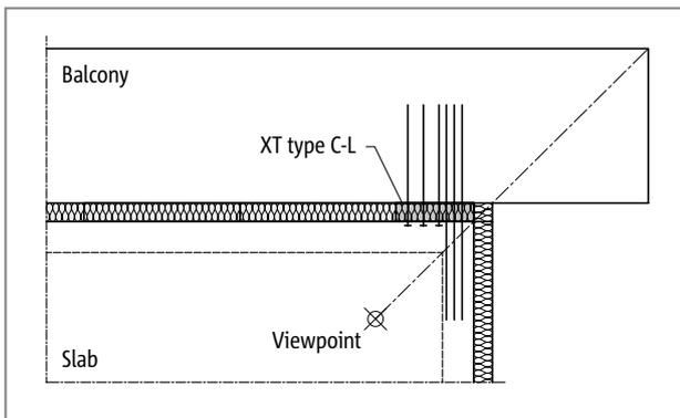
Fig. 55: Schöck Isokorb® XT type C: Balcony projecting over corner of building (application XT type C-L)
