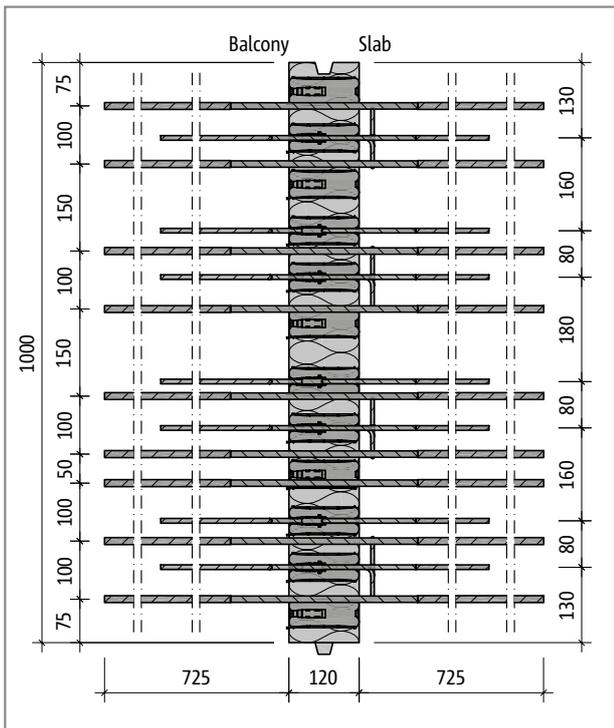
Fig. 35: Schöck Isokorb® XT type K-M8: Product plan view
