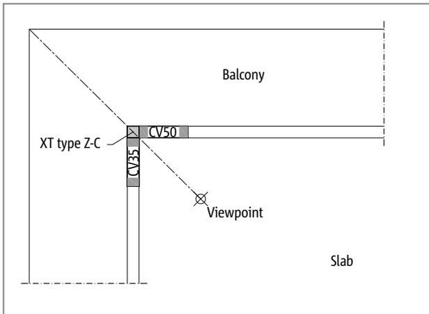
Fig. 49: Schöck Isokorb® XT type C: Concrete cover selectable: Here CV35 left from viewpoint, concrete cover CV50 right from viewpoint
