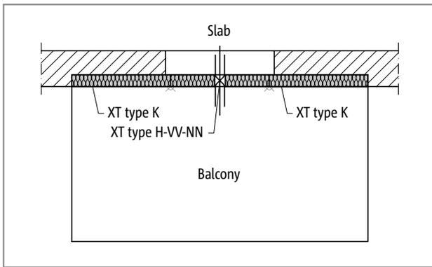
Fig. 173: Schöck Isokorb® XT type H: Balcony freely cantilevered
