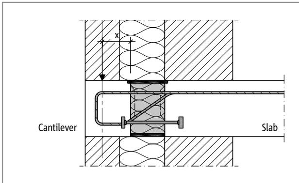
Fig. 246: Schöck Isokorb® XT type O: Corbel with faced masonry
