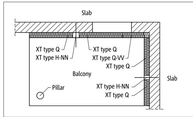
Fig. 174: Schöck Isokorb® XT type H: Balcony supported on two sides using columns
