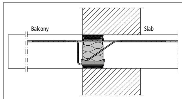
Fig. 23: Schöck Isokorb® XT type K: Connection with single-leaf masonry
