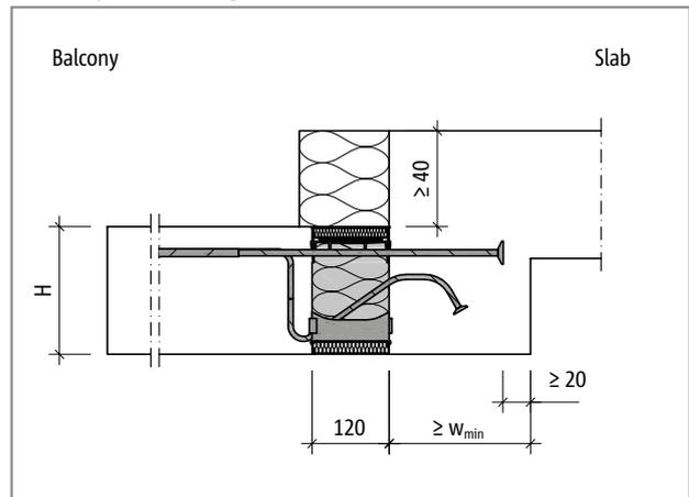
Fig. 90: Schöck Isokorb® XT type K-U: Balcony with height offset downwards and external insulation
