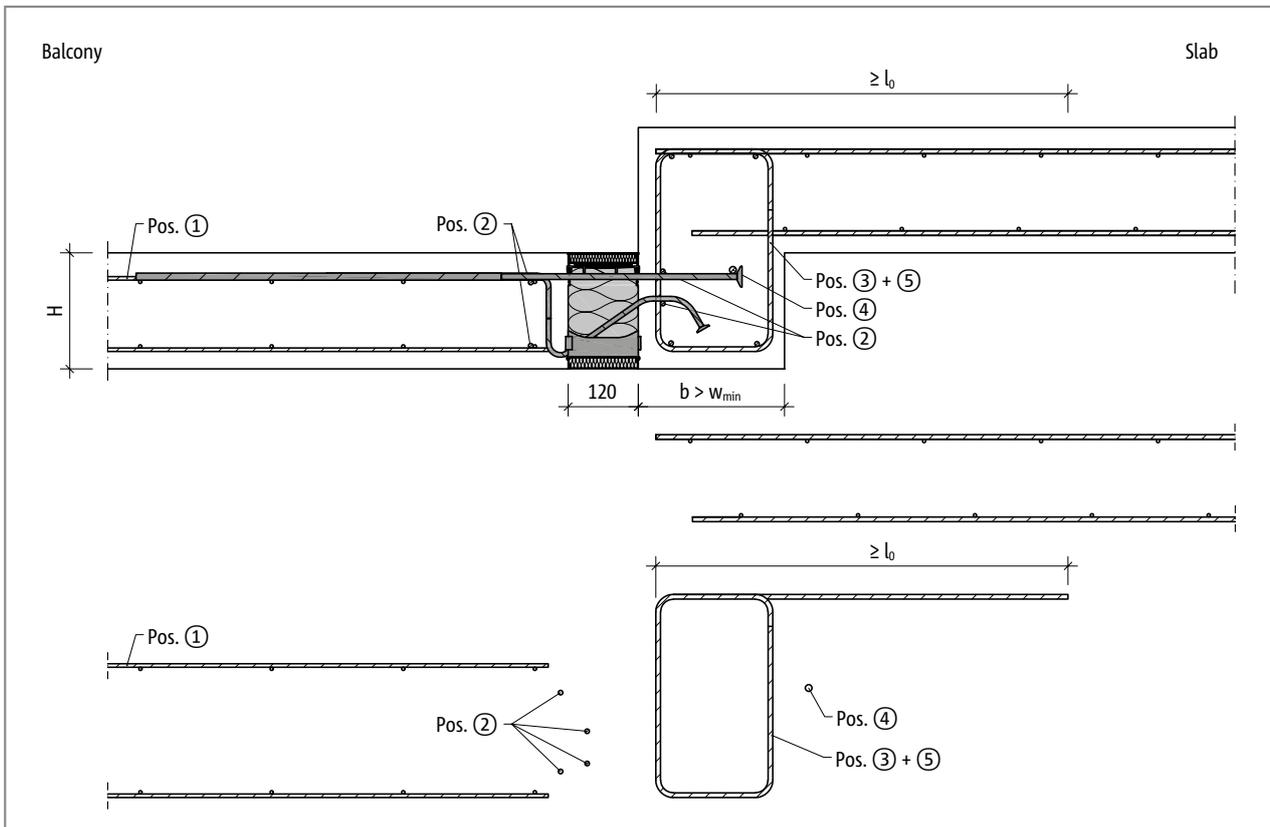
Fig. 110: Schöck Isokorb® XT type K-U: On-site reinforcement for balcony with height offset downwards with larger structural element dimension ( $w_{vorh} > w_{min}$ )
