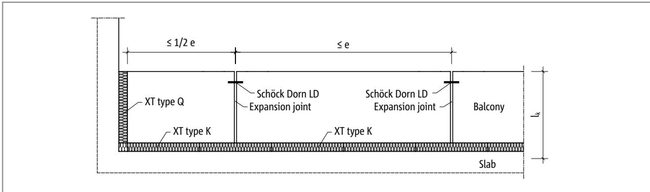
Fig. 28: Schöck Isokorb® XT type K: Expansion joint arrangement
