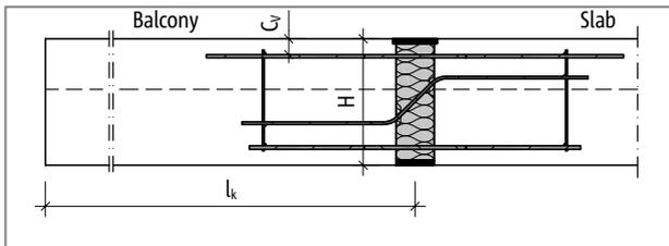
Fig. 260: Schöck Isokorb® XT type B: Static system
