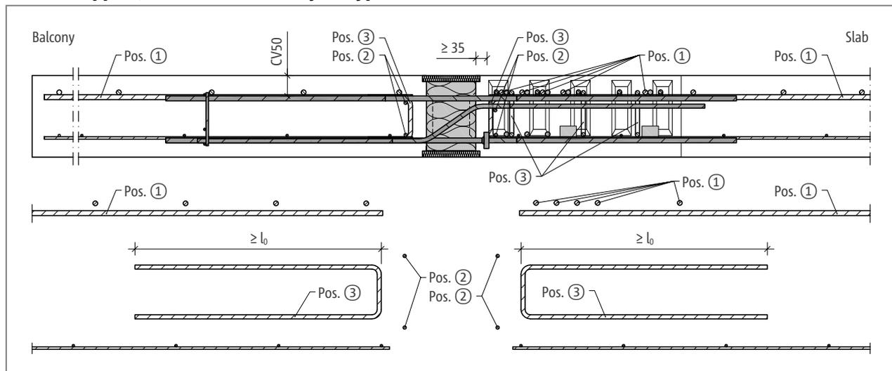
Fig. 71: Schöck Isokorb® XT type C: On-site reinforcement outer corner (section XT type C-L-CV50, view XT type C-R-CV35)
