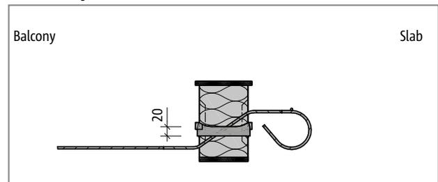
Fig. 8: Schöck Isokorb® XT type Q-V1 to V4: Product section
