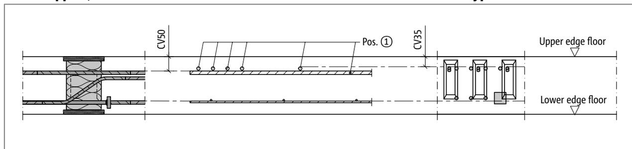
The reinforcement in the reinforced concrete slab is determined from the structural engineer's design. With this both the effective moment and the effective shear force should be taken into account.
