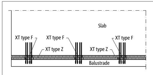
Fig. 235: Schöck Isokorb® XT type F, Z: Frontally attached balustrades
