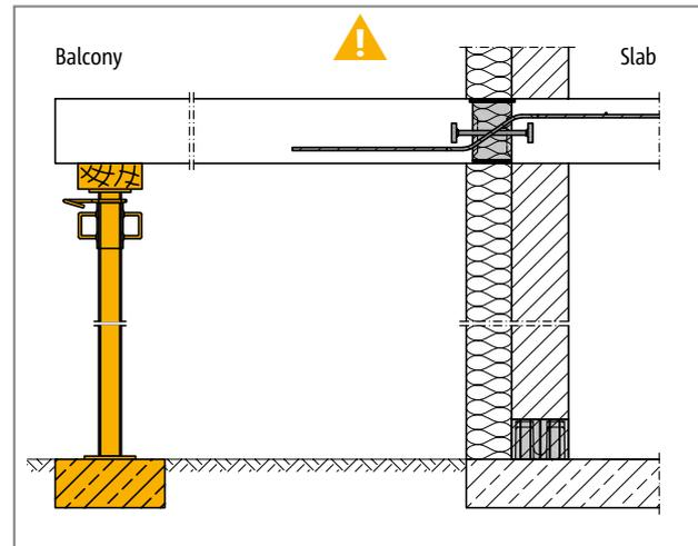
Fig. 170: Schöck Isokorb® XT type Q-P: Continuous support required
