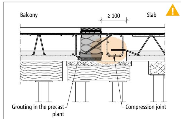
Fig. 44: Schöck Isokorb® XT type K: Indirect support, installation in conjunction with element slabs (here:  $h \leq 180$  mm), compression joint on floor side
