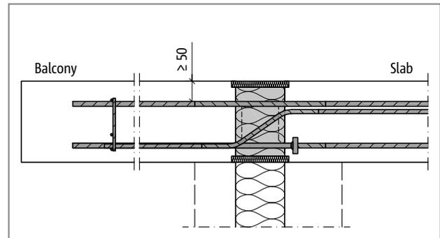
Fig. 58: Schöck Isokorb® XT type C-CV50: Connection with non-load-bearing cavity wall masonry
