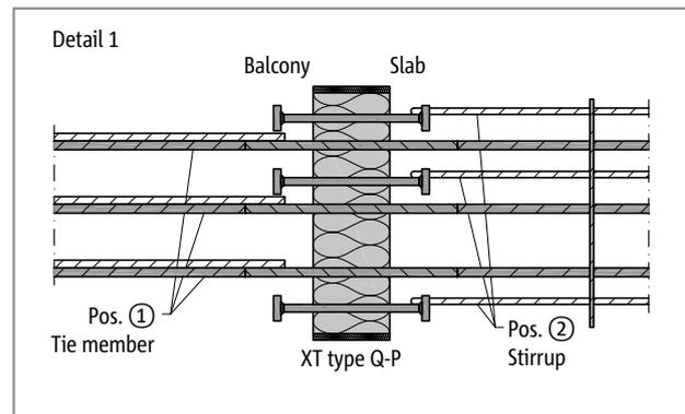
Fig. 168: Schöck Isokorb® XT type Q-P, Q-PZ: Detail 1; Reinforcement connection tie member
