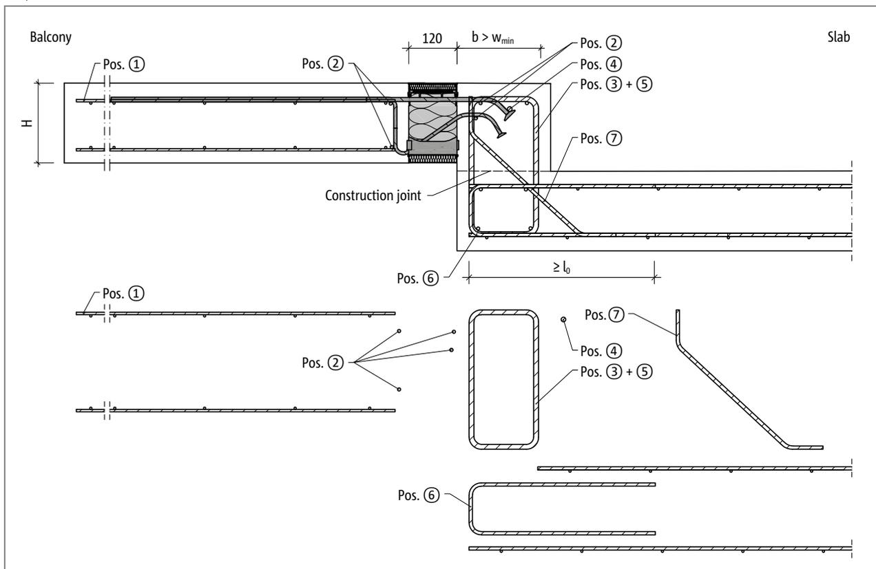
Fig. 114: Schöck Isokorb® XT type K-O: On-site reinforcement for balcony with height offset upwards with larger structural element dimension ( $w_{vorh} > w_{min}$ )
