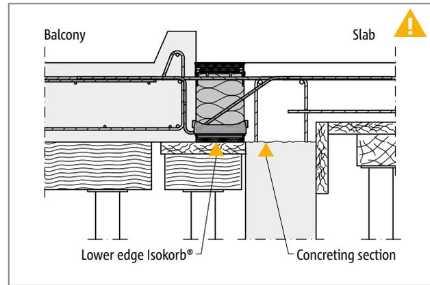
Fig. 42: Schöck Isokorb® XT type K: Fully finished balcony with height offset floor on precast reinforced concrete wall
