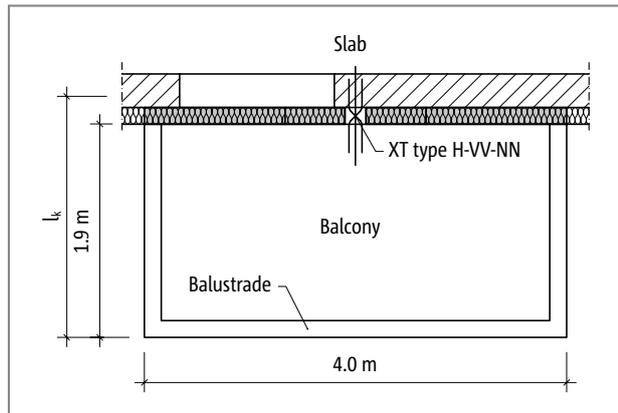
Fig. 190: Schöck Isokorb® XT type K, H: Plan view
