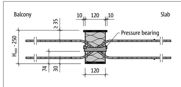
Fig. 137: Schöck Isokorb® XT type Q-VV5 to Q-VV8: Product section
