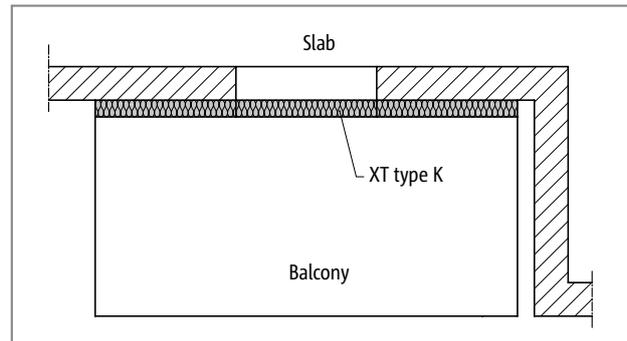
Fig. 19: Schöck Isokorb® XT type K: Balcony with facade offset
