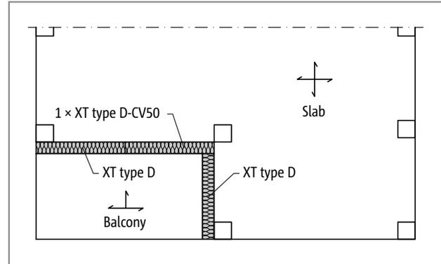
Fig. 205: Schöck Isokorb® XT type D: Two-way spanning
