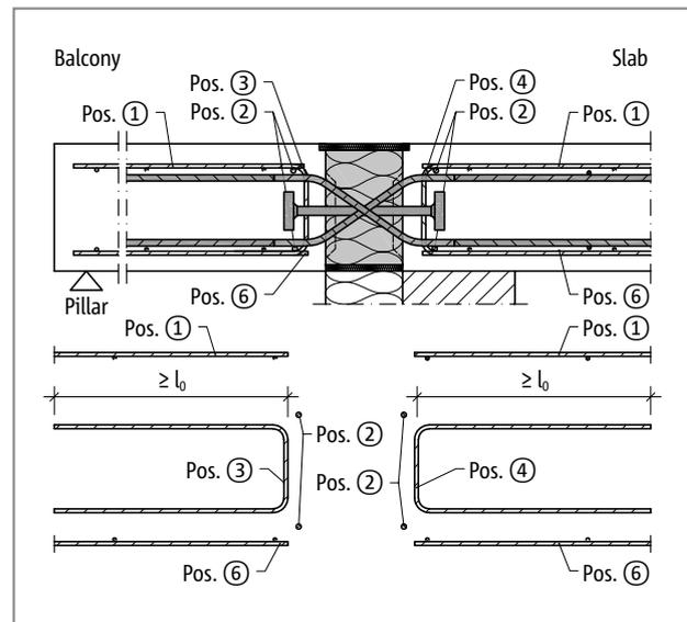
Fig. 166: Schöck Isokorb® XT type Q-P-VV: On-site reinforcement
