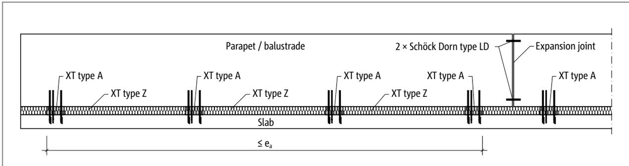
Fig. 221: Schöck Isokorb® XT type A: Expansion joint arrangement
