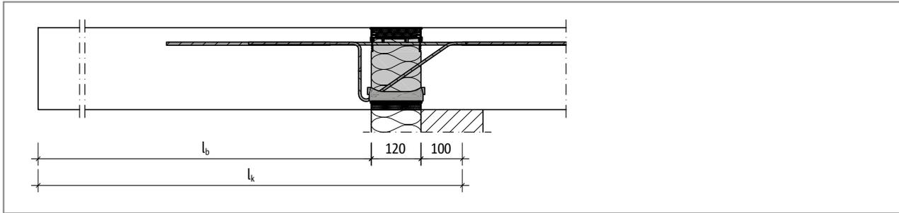
Fig. 9: Schöck Isokorb® XT type K: System cantilever length ( $l_k$ ) for design and geometric cantilever ( $l_b$ )
