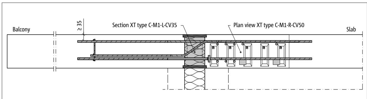
Fig. 59: Schöck Isokorb® XT type C: Outer corner with non-load-bearing cavity wall masonry (section XT type C-L-CV35; view XT type C-R-CV50)
