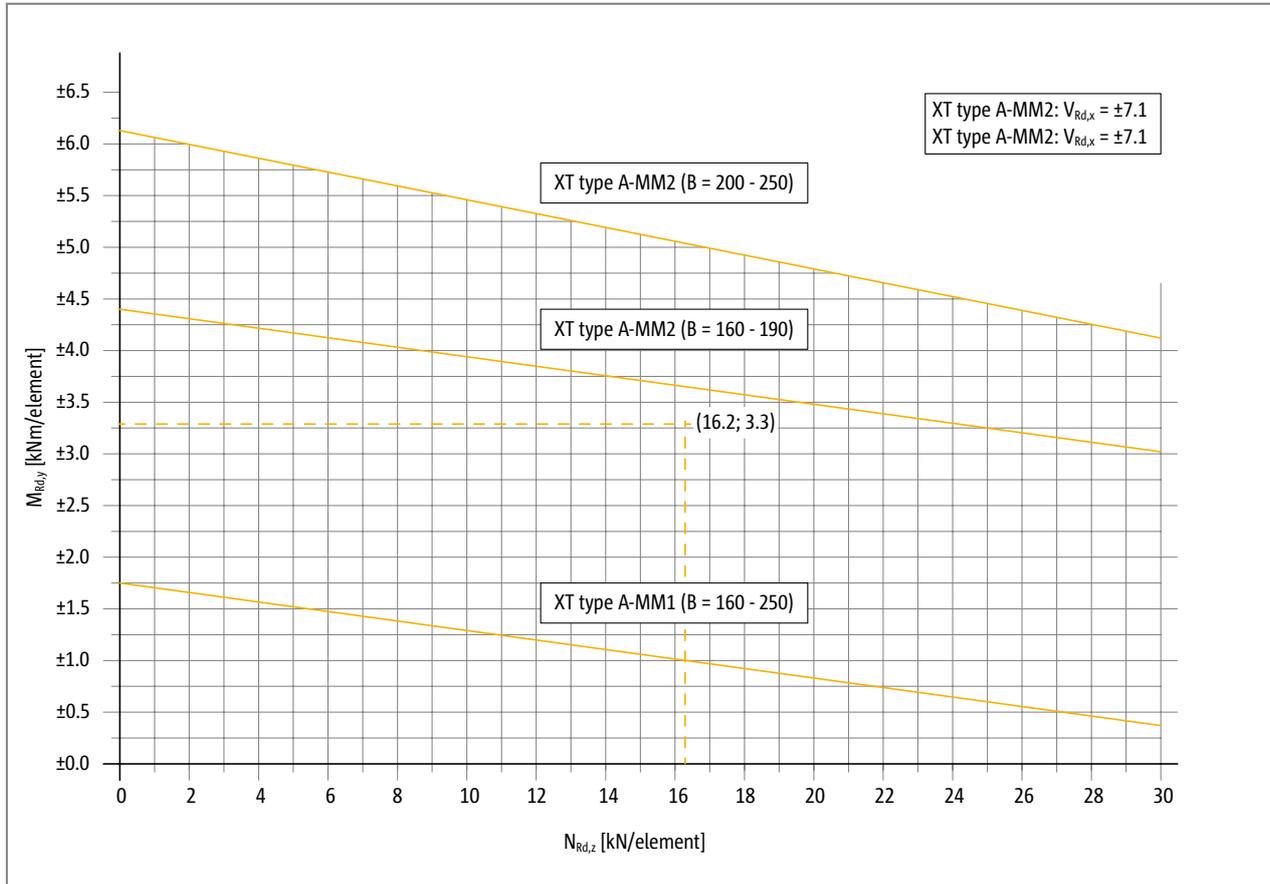
The point  $((N_{Ed,z}; M_{Ed,y}) = (16.2 \text{ kN}; 3.3 \text{ kNm})$  lies below the line of the Schöck Isokorb® XT type A-MM2 (B = 200 - 250).
