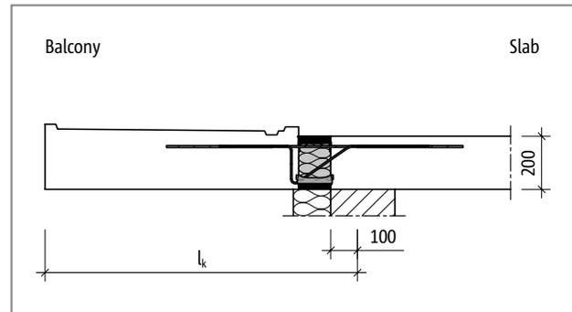
Fig. 46: Schöck Isokorb® XT type K: Static system
