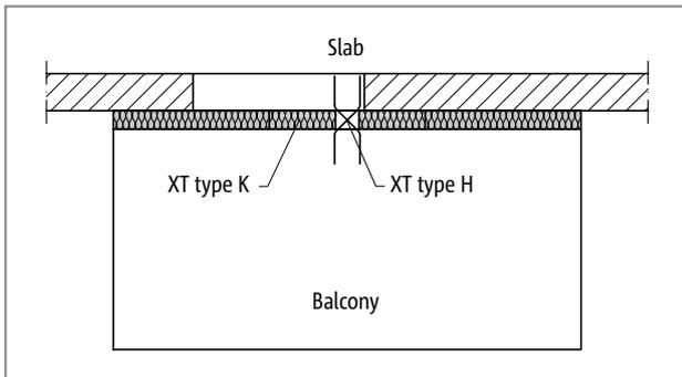
Fig. 18: Schöck Isokorb® XT type K: Balcony freely cantilevered; optional with XT type H (from page 125) with planned horizontal loads (e. g. closed ballustrades)
