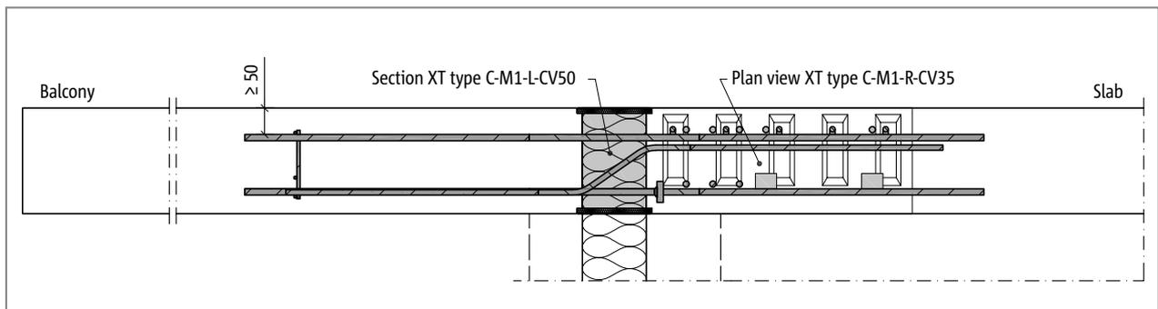
Fig. 60: Schöck Isokorb® XT type C: Outer corner with non-load-bearing cavity wall masonry (view XT type C-L-CV50; section XT type C-R-CV35)
