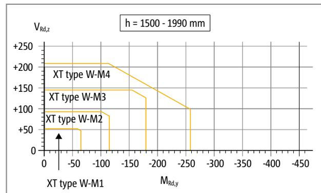
Fig. 269: Schöck Isokorb® XT type W: Interaction diagram
