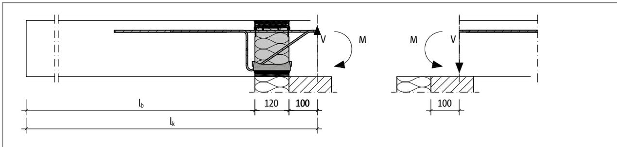
Fig. 11: Schöck Isokorb® XT type K: Determined design stress resultants applied to floor slab
