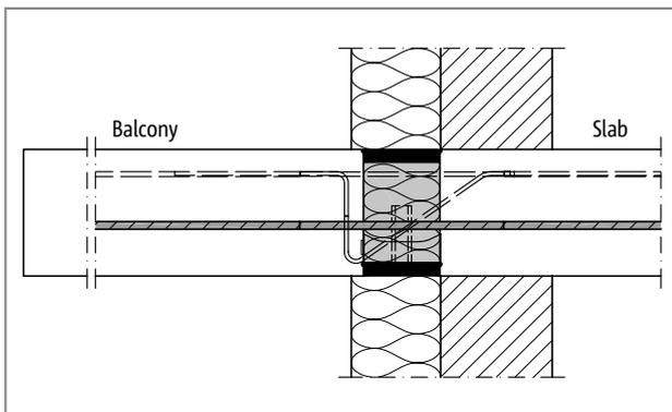
Fig. 175: Schöck Isokorb® XT type K, H-NN: Masonry with external insulation
