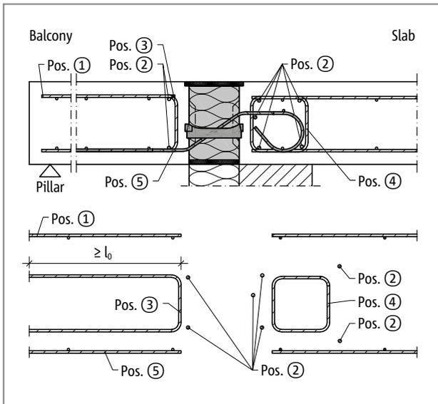
Fig. 142: Schöck Isokorb® XT type Q-V1 to V4: On-site reinforcement
