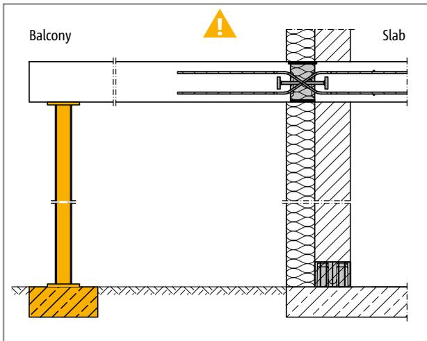
Fig. 169: Schöck Isokorb® XT type Q-P-VV: Continuous support required
