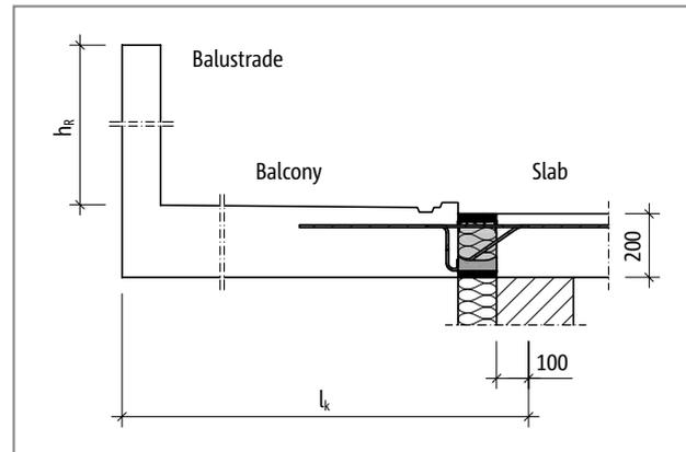
Fig. 191: Schöck Isokorb® XT type K: Static system
