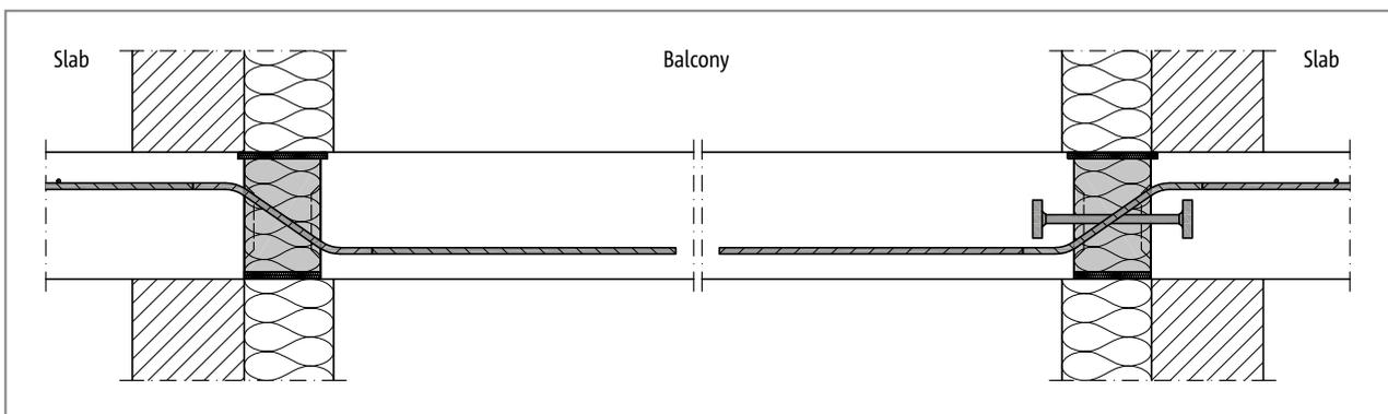
Fig. 154: Schöck Isokorb® XT type Q-P, Q-PZ: Application case recessed balcony see p. 119
