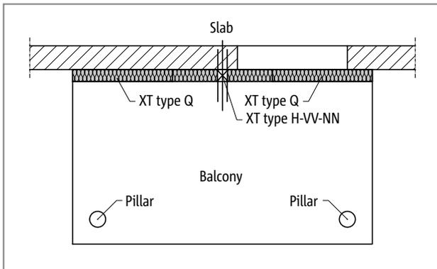
Fig. 171: Schöck Isokorb® XT type H: Balcony with column support
