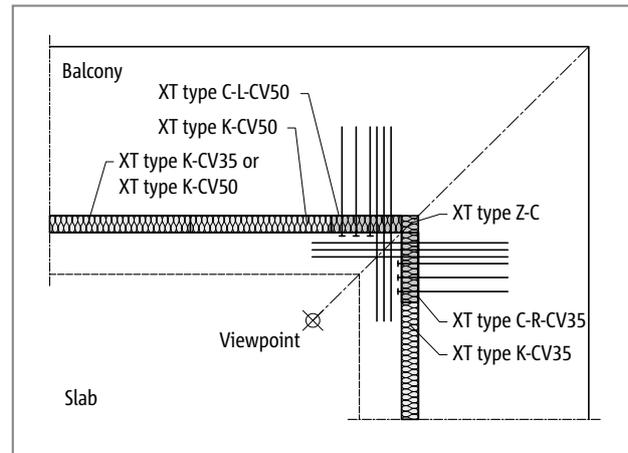
Fig. 54: Schöck Isokorb® XT type C: Balcony with outer corner freely cantilevered (application XT type C-L-CV50, XT type C-R-CV35)
