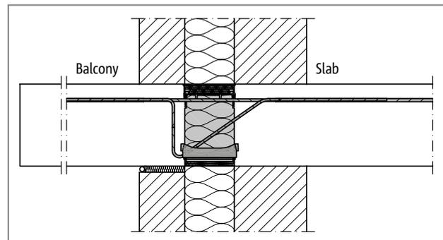
Fig. 25: Schöck Isokorb® XT type K: Cavity wall with a balcony at inner slab level
