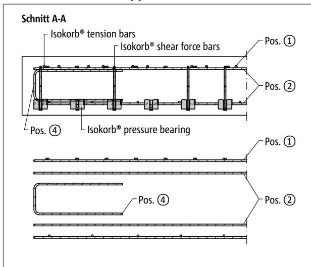
Fig. 39: Schöck Isokorb® XT type K: On-site reinforcement balcony side in section A-A; Pos. 4 = side reinforcement on the free edge perpendicular to the Schöck Isokorb
