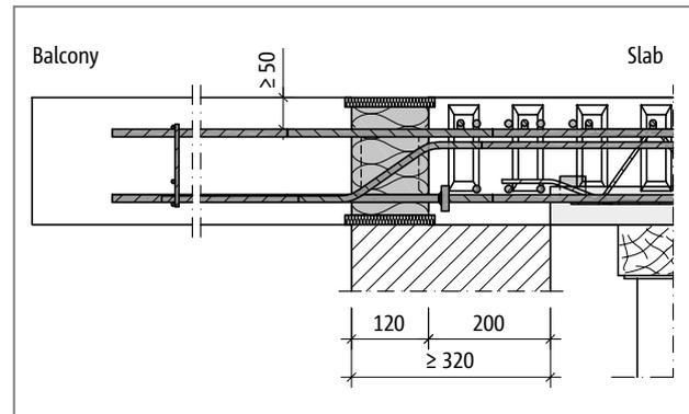
Fig. 77: Schöck Isokorb® XT type C: Prefabricated slab with edge support with thermal insulating masonry (section XT type C-R-CV50, view XT type C-L-CV35)
