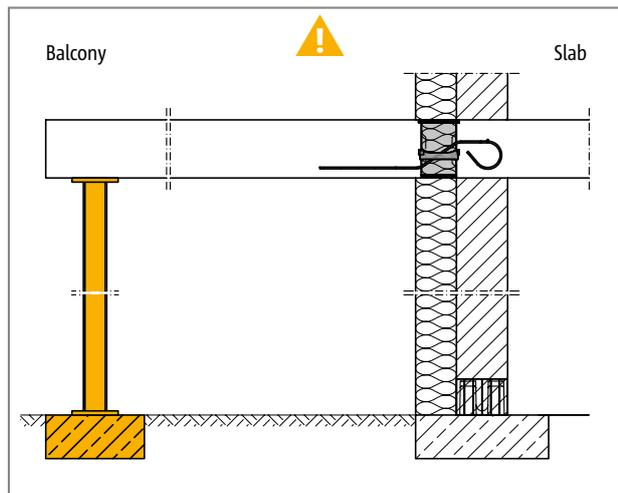
Fig. 149: Schöck Isokorb® XT type Q: Continuous support required
