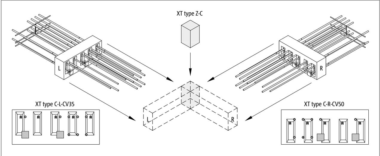
Fig. 51: Schöck Isokorb® XT type C-L-CV35, XT type C-R-CV50: Arrangement at the corner using corner insulating element
