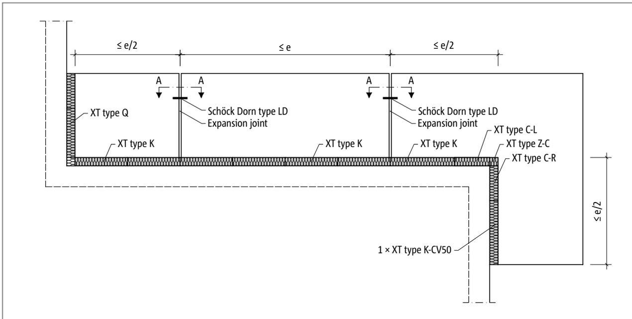
Fig. 15: Schöck Isokorb® XT type K: Expansion joint spacing longitudinally displaceable shear force dowel, e. g. Schöck dowel
