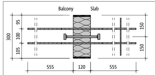
Fig. 160: Schöck Isokorb® XT type Q-P-V1: Product plan view
