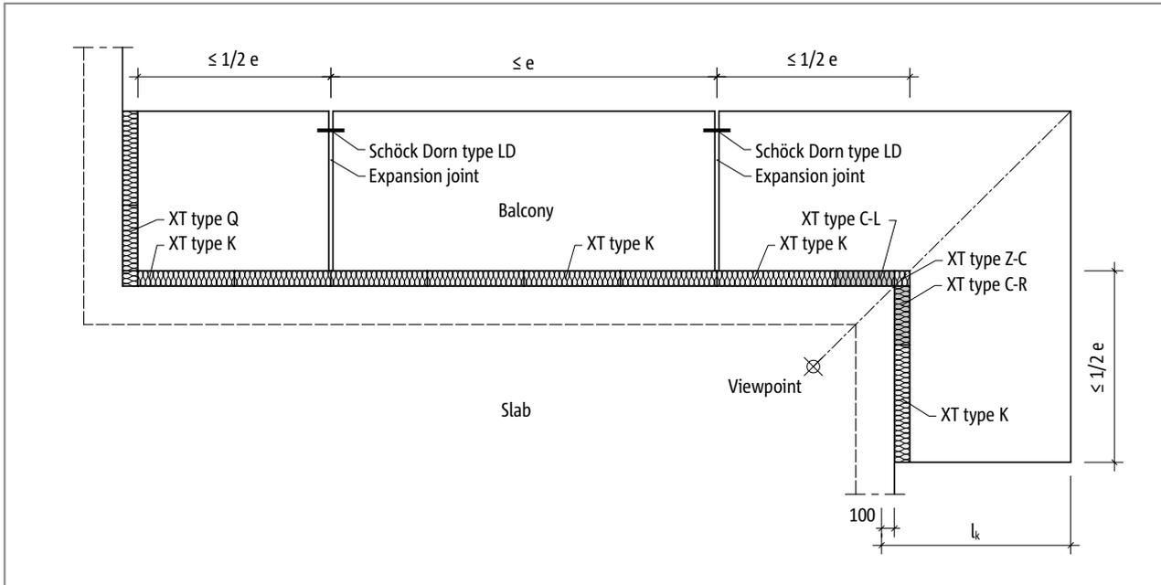
Fig. 63: Schöck Isokorb® XT type C: Expansion joint arrangement
