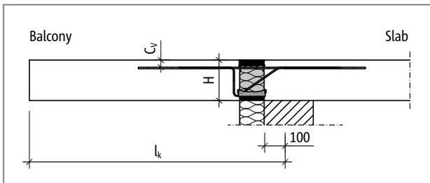
Fig. 27: Schöck Isokorb® XT type K: Static system
