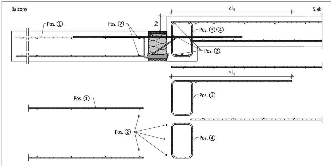
Fig. 108: Schöck Isokorb® XT type K: On-site reinforcement for small height offset
