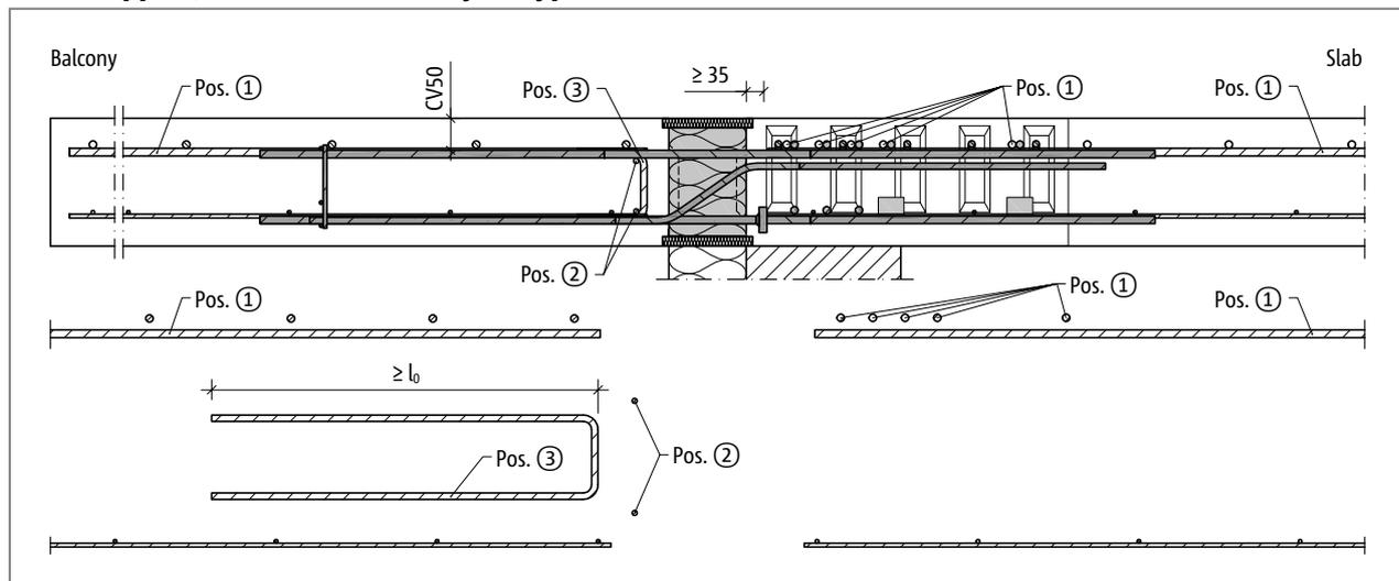
Fig. 73: Schöck Isokorb® XT type C: On-site reinforcement outer corner (section XT type C-L-CV50, view XT type C-R-CV35)
