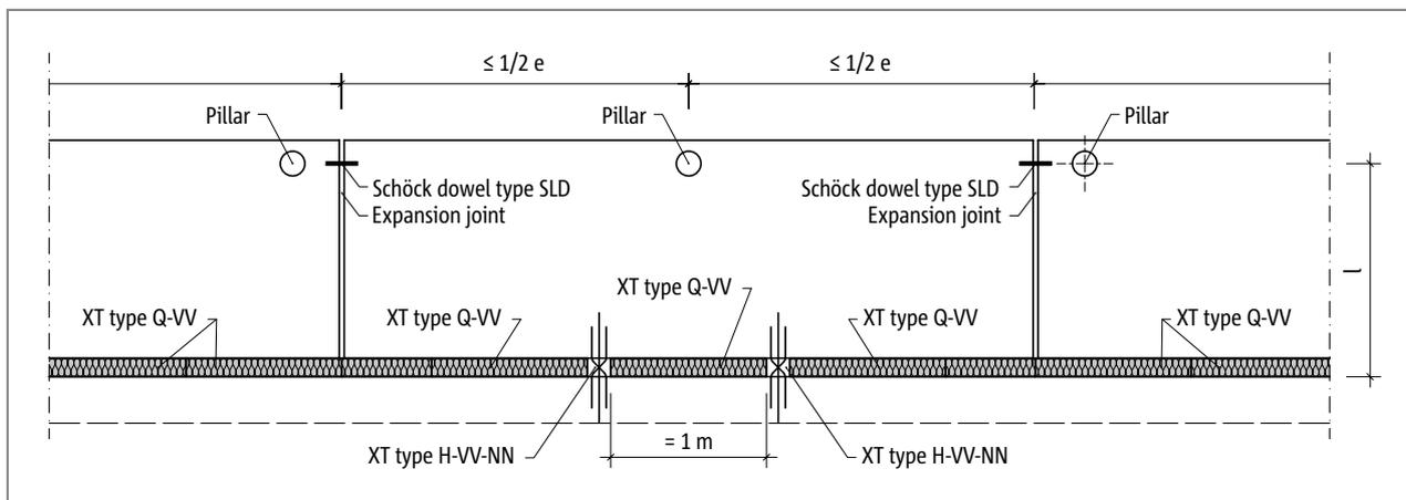
Fig. 180: Schöck Isokorb® XT type H: Expansion joint arrangement
