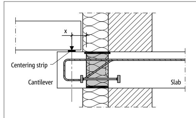
Fig. 247: Schöck Isokorb® XT type O: Connection of a console as floor support; centring battens prevent a displacement of the load application point
