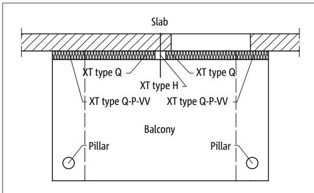
Fig. 153: Schöck Isokorb® XT type Q-P-VV, Q: Balcony with column support with various bearing stiffnesses; optionally with XT type H for transmission of ordinary horizontal force
