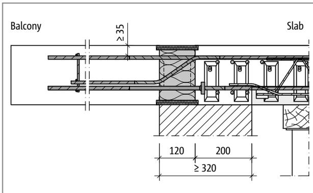
Fig. 76: Schöck Isokorb® XT type C: Prefabricated slab with edge support with thermal insulating masonry (section XT type C-L-CV35, view XT type C-R-CV50)
