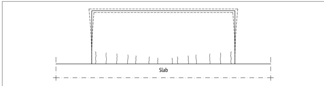
Fig. 12: Balcony slab without Schöck Isokorb®: Crack formation through fatigue possible
