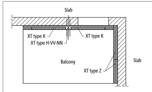
Fig. 172: Schöck Isokorb® XT type H: Balcony freely cantilevered
