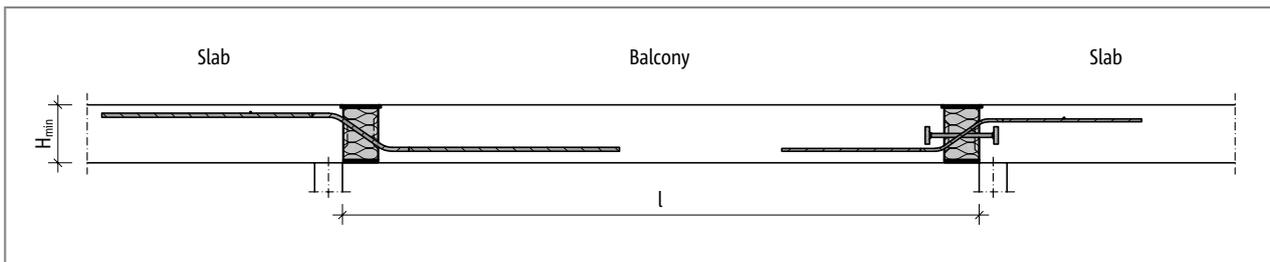
Fig. 156: Schöck Isokorb® XT type Q-PZ, Q-P: Static system
