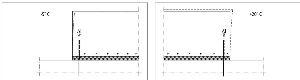
Fig. 13: Schöck Isokorb®: Displacement of the outer bars of a balcony slab by  $\Delta l$  as a result of temperature deformation
