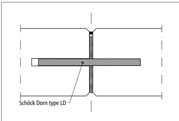
Fig. 16: Schöck Dorn: Expansion joint formation in in-situ concrete
