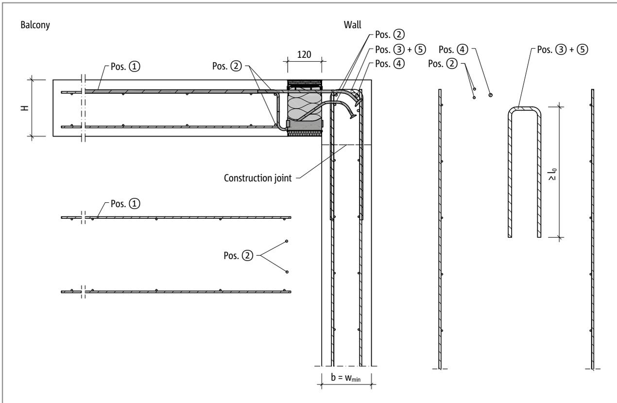
Fig. 115: Schöck Isokorb® XT type K-O: On-site reinforcement for wall connection upwards with minimum structural element dimension ( $w_{vorh} = w_{min}$ )
