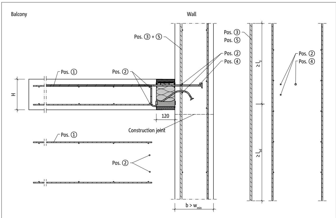
Fig. 112: Schöck Isokorb® XT type K-U: On-site reinforcement for wall connection upwards with larger structural element dimension ( $w_{vorh} > w_{min}$ )
