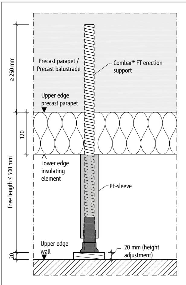
Fig. 229: Schöck Combar® FT erection support: planning dimensions
