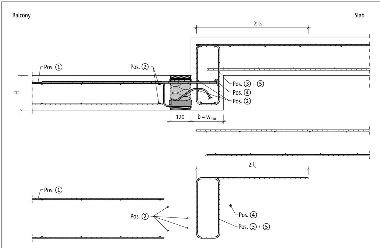
Fig. 109: Schöck Isokorb® XT type K-U: On-site reinforcement for balcony with height offset downwards with minimum structural element dimension ( $w_{vorh} = w_{min}$ )
