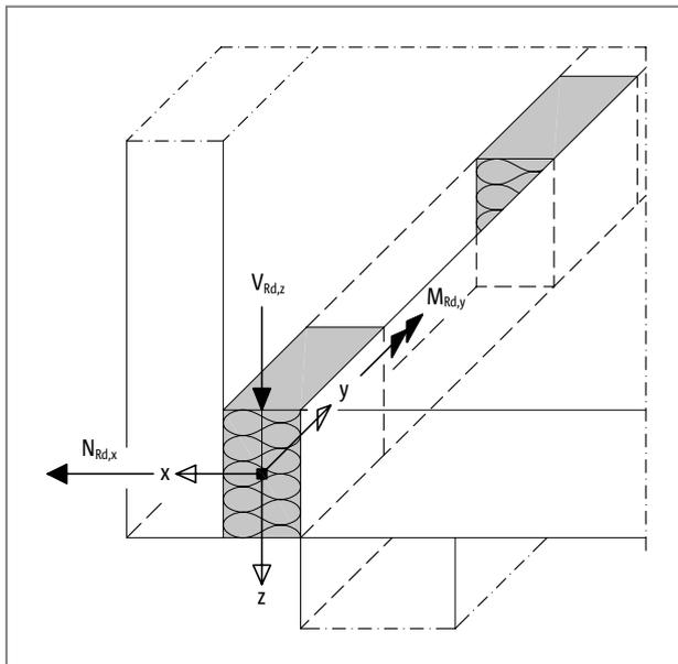
Fig. 238: Schöck Isokorb® XT type F: Sign convention for the design
