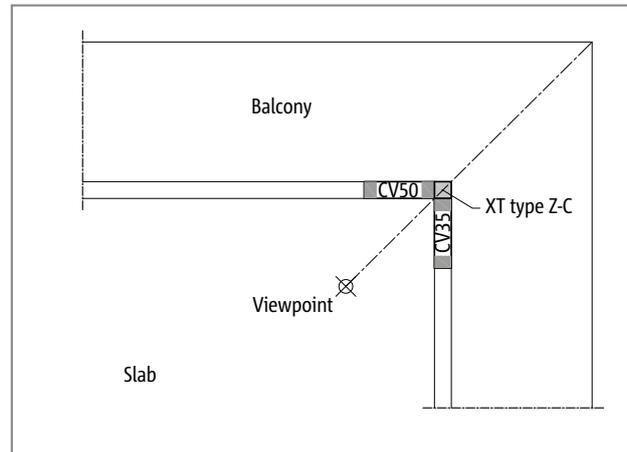
Fig. 50: Schöck Isokorb® XT type C: Concrete cover selectable: Here CV50 left from viewpoint, concrete cover CV35 right from viewpoint
