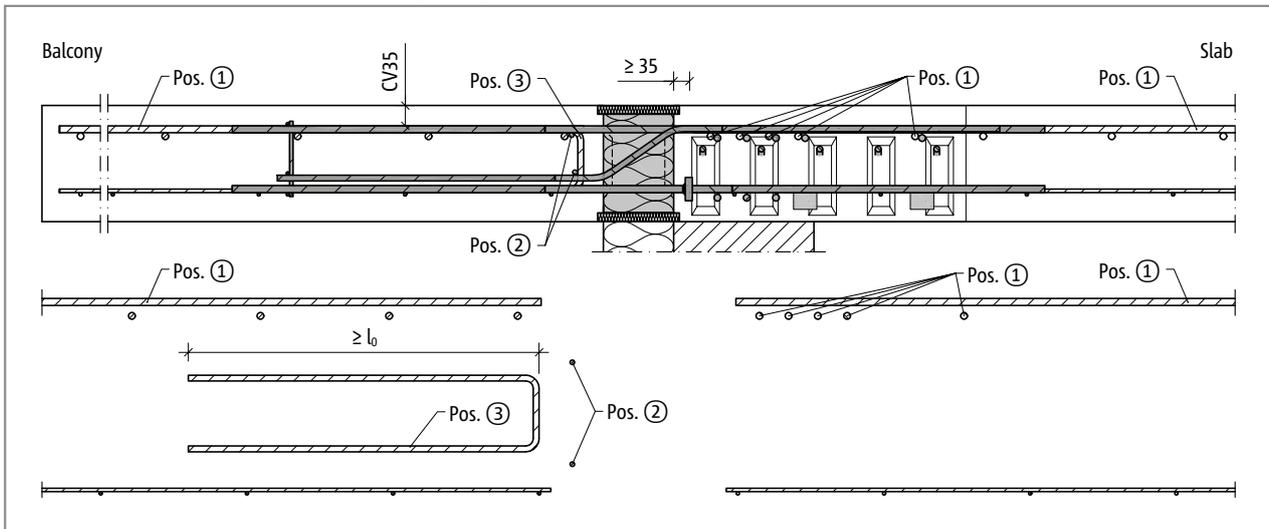
Fig. 72: Schöck Isokorb® XT type C: On-site reinforcement outer corner balcony (section XT type C-L-CV35, view XT type C-R-CV50)
