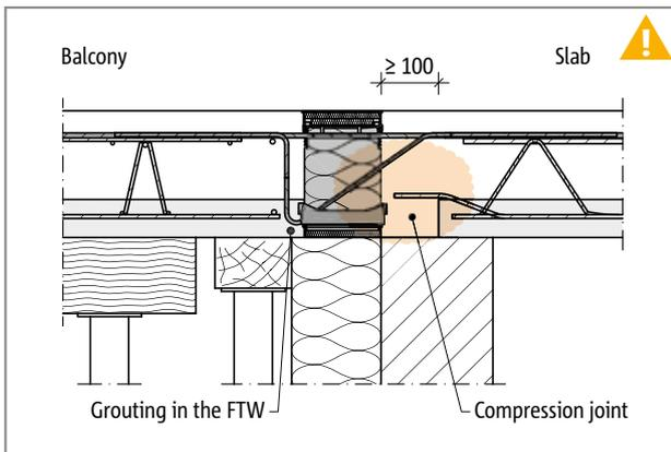
Fig. 43: Schöck Isokorb® XT type K: Direct support, installation in conjunction with element slabs (here:  $h \leq 180$  mm), compression joint on floor side
