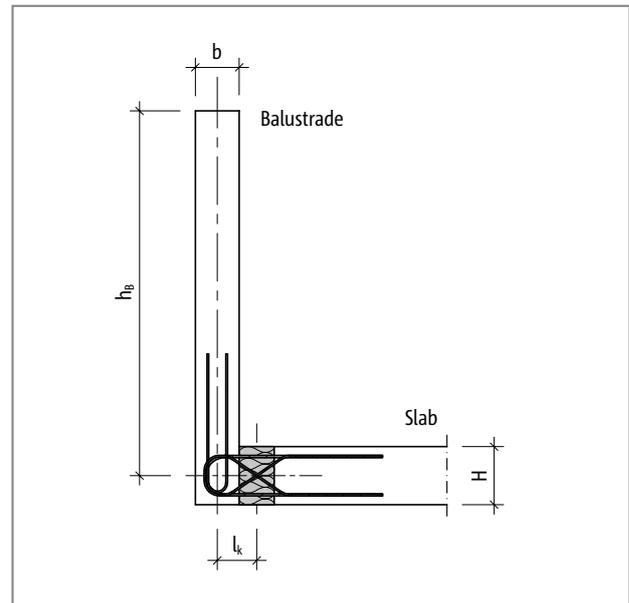
Fig. 239: Schöck Isokorb® XT type F: Static system
