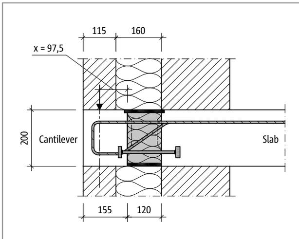
Fig. 255: Schöck Isokorb® XT type O: Wall construction for design example
