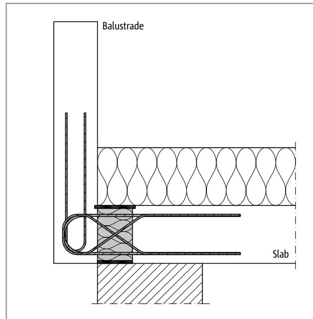
Fig. 237: Schöck Isokorb® XT type F: Connection of a frontally attached balustrade with thermal insulating masonry
