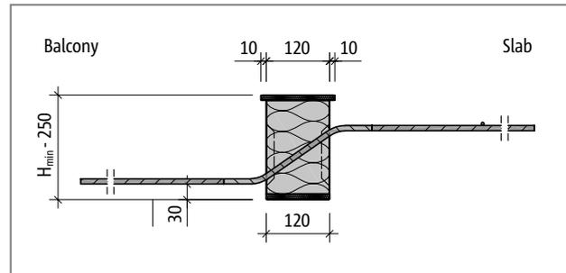
Fig. 139: Schöck Isokorb® XT type Q-Z-V5 to Q-Z-V8: Product section
