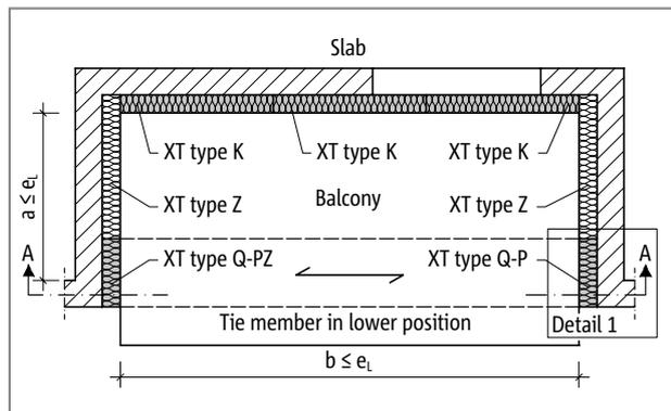
Fig. 167: Schöck Isokorb® XT type Q-PZ, Q-P: Plan view recessed balcony
