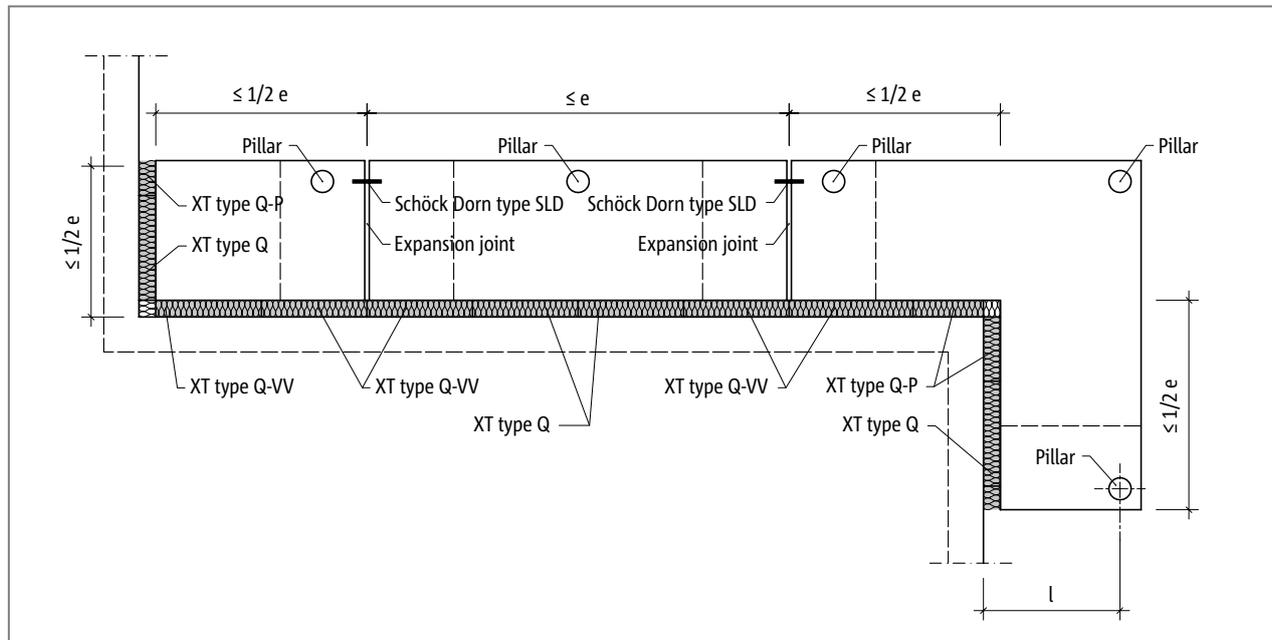
Fig. 158: Schöck Isokorb® XT type Q-P, Q-P-VV: Expansion joint arrangement
