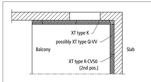
Fig. 21: Schöck Isokorb® XT type K, Q-VV: balcony with inner corner, supported two-sided
