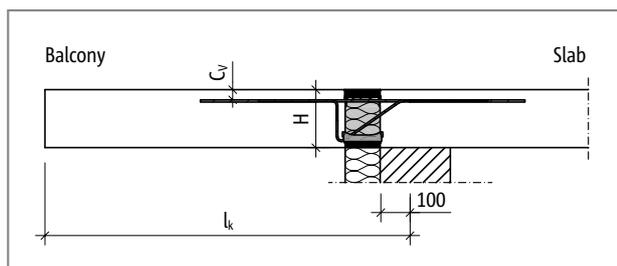
Fig. 26: Schöck Isokorb® XT type K: Static system
