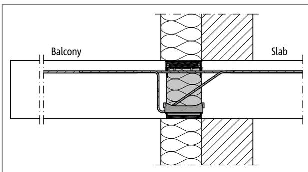
Fig. 22: Schöck Isokorb® XT type K: Connection with thermal insulation composite system (TICS)
