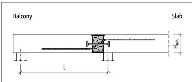
Fig. 155: Schöck Isokorb® XT type Q-P: Static system
