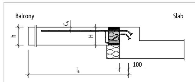
Fig. 96: Schöck Isokorb® XT type K-O: Static system
