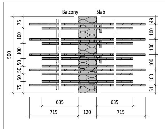
Fig. 69: Schöck Isokorb® XT type C-R-M2-V2: Product plan view
