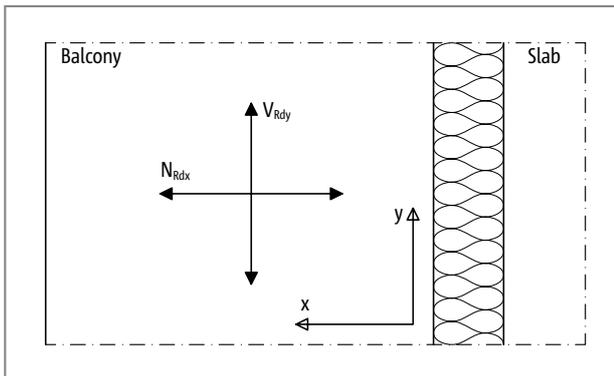
Fig. 178: Schöck Isokorb® XT type H: Sign rule for the design
