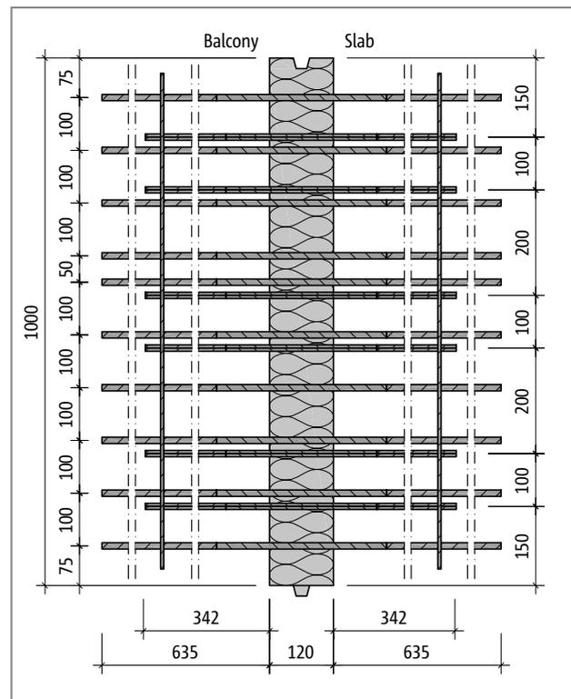
Fig. 212: Schöck Isokorb® XT type D-MM4-VV1: Plan view
