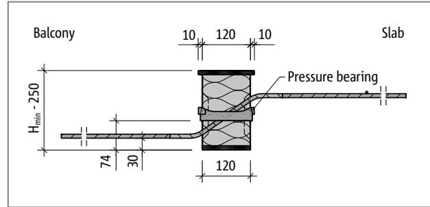
Fig. 135: Schöck Isokorb® XT type Q-V5 to Q-V8: Product section
