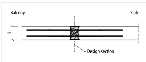
Fig. 208: Schöck Isokorb® XT type D: Static system
