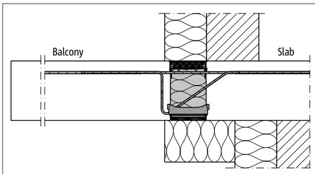
Fig. 24: Schöck Isokorb® XT type K: Connection for indirectly positioned floor and TICS
