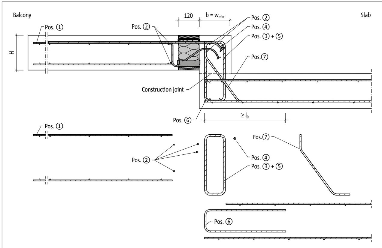
Fig. 113: Schöck Isokorb® XT type K-O: On-site reinforcement for balcony with height offset upwards with minimum structural element dimension ( $w_{vorh} = w_{min}$ )
