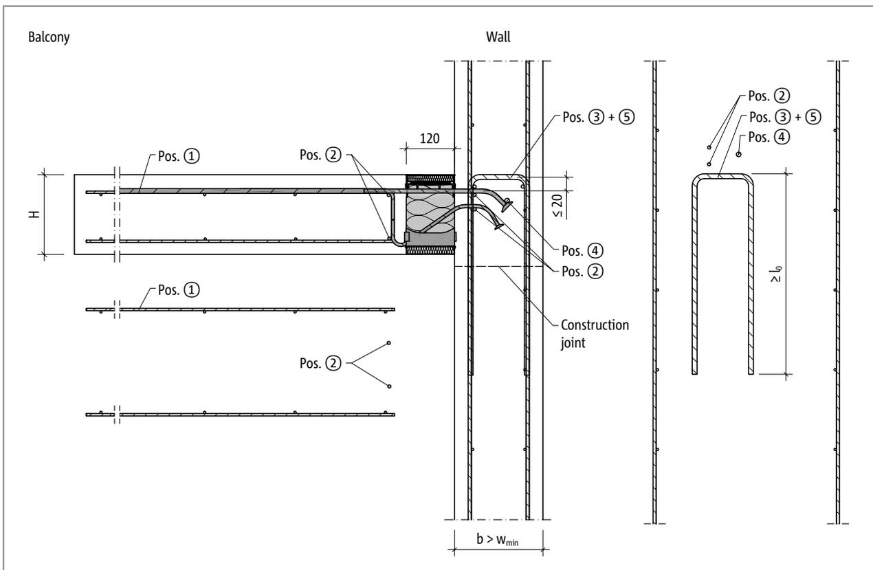
Fig. 116: Schöck Isokorb® XT type K-O: On-site reinforcement for wall connection with larger structural element dimension ( $w_{vorh} > w_{min}$ )
