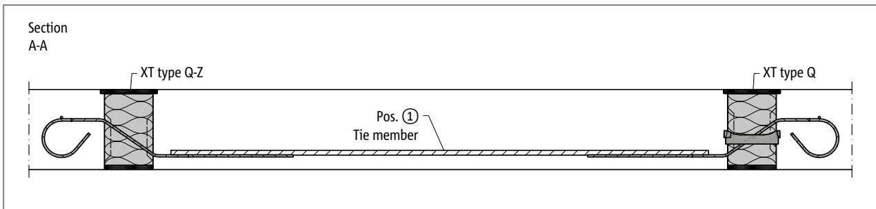
Fig. 147: Schöck Isokorb® XT type Q-Z-V1 to Q-Z-V4, Q-V1 to Q-V4: Section A-A; one direction spanned reinforced concrete slab
