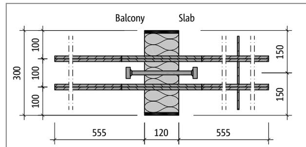
Fig. 162: Schöck Isokorb® XT type Q-P-VV1: Product plan view
