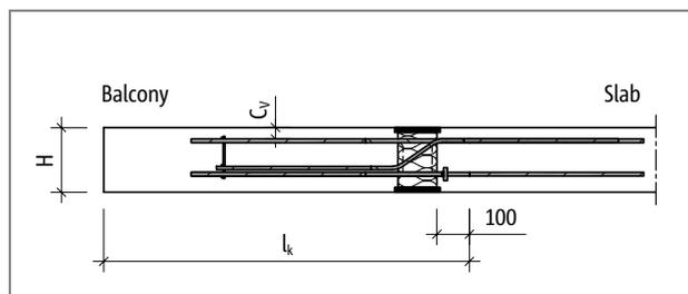
Fig. 61: Schöck Isokorb® XT type C: Static system
