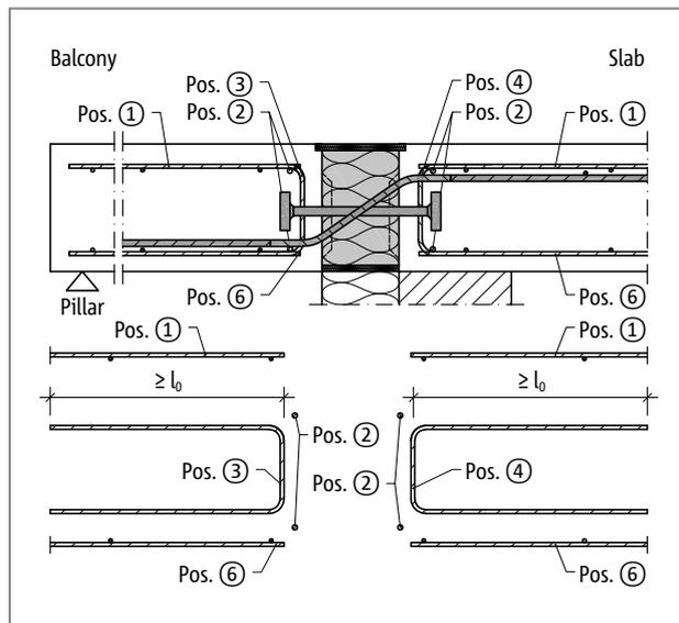
Fig. 165: Schöck Isokorb® XT type Q-P: On-site reinforcement
