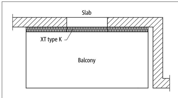
Fig. 45: Schöck Isokorb® XT type K: Plan view
