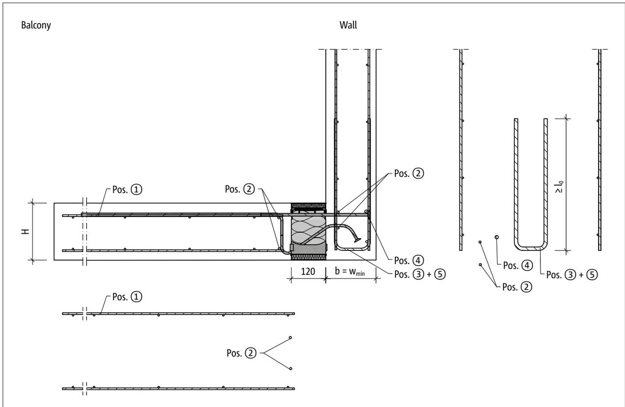
Fig. 111: Schöck Isokorb® XT type K-U: On-site reinforcement for wall connection upwards with minimum structural element dimension ( $w_{vorh} = w_{min}$ )
