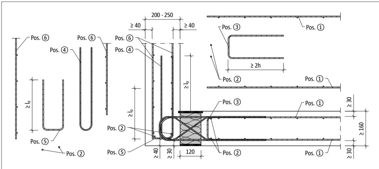
Fig. 244: Schöck Isokorb® XT type F: On-site reinforcement with parapet/balustrade width  $b = 200 - 250$ ; on-site reinforcement  $b = 160 - 190$  such as  $b = 200 - 250$  without Pos. 5
