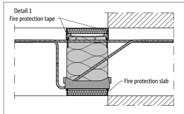
Fig. 2: Schöck Isokorb® XT type K with REI120: Detail 1
