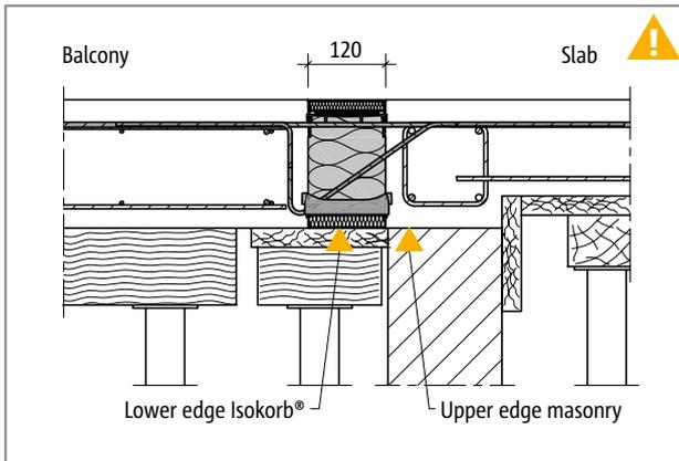
Fig. 41: Schöck Isokorb® XT type K: In-situ concrete balcony with height offset floor on masonry wall
