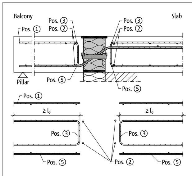
Fig. 144: Schöck Isokorb® XT type Q-V5 to Q-V8: On-site reinforcement
