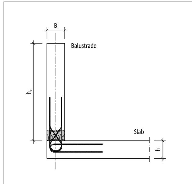
Fig. 219: Schöck Isokorb® XT type A: Static system
