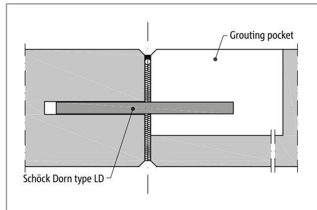
Fig. 17: Schöck Dorn: Expansion joint formation precast concrete balcony
