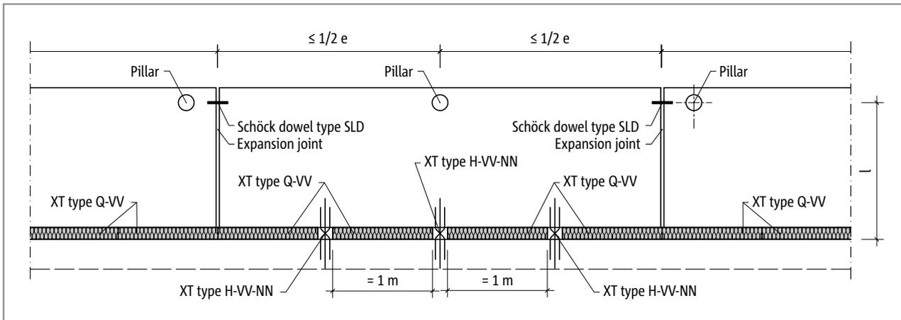
Fig. 181: Schöck Isokorb® XT type H: Expansion joint arrangement
