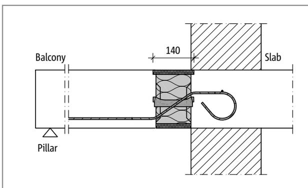
Fig. 3: Schöck Isokorb® XT type Q with REI120: Fire protection board top projecting laterally
