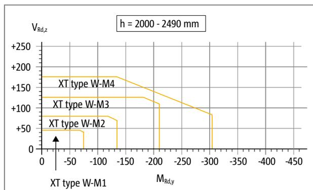
Fig. 270: Schöck Isokorb® XT type W: Interaction diagram
