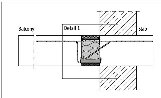
Fig. 1: Schöck Isokorb® XT type K with REI120: Fire protection boards top and bottom; laterally integrated fire protection strips
