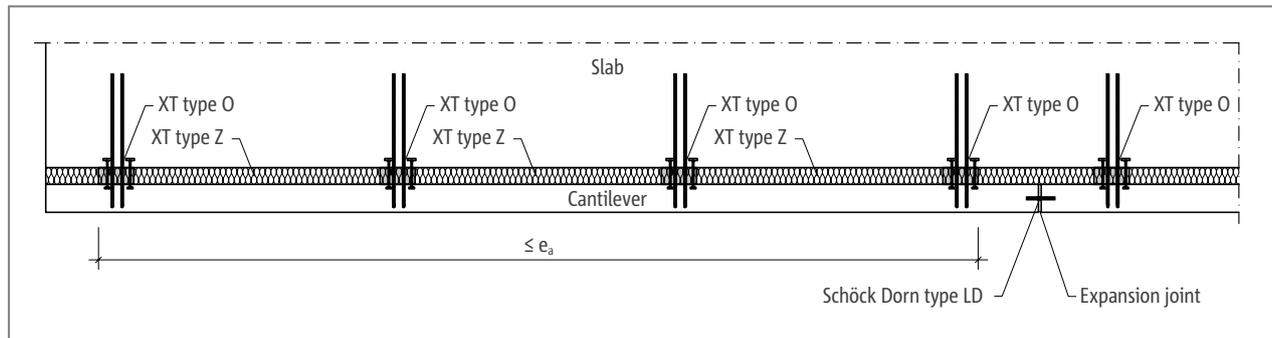
Fig. 250: Schöck Isokorb® XT type O: Expansion joint arrangement
