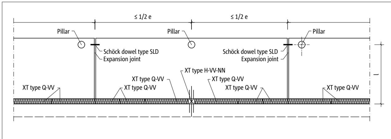
Fig. 179: Schöck Isokorb® XT type H: Expansion joint arrangement
