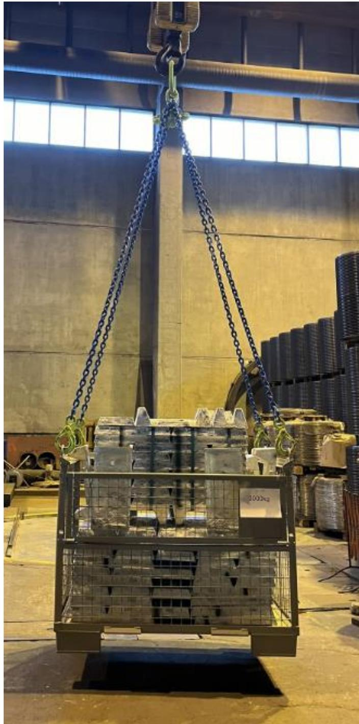
Picture from Stacking and loading test with 2 x nominal load in the upper Erobox (2000 kg) – no instability detected.
