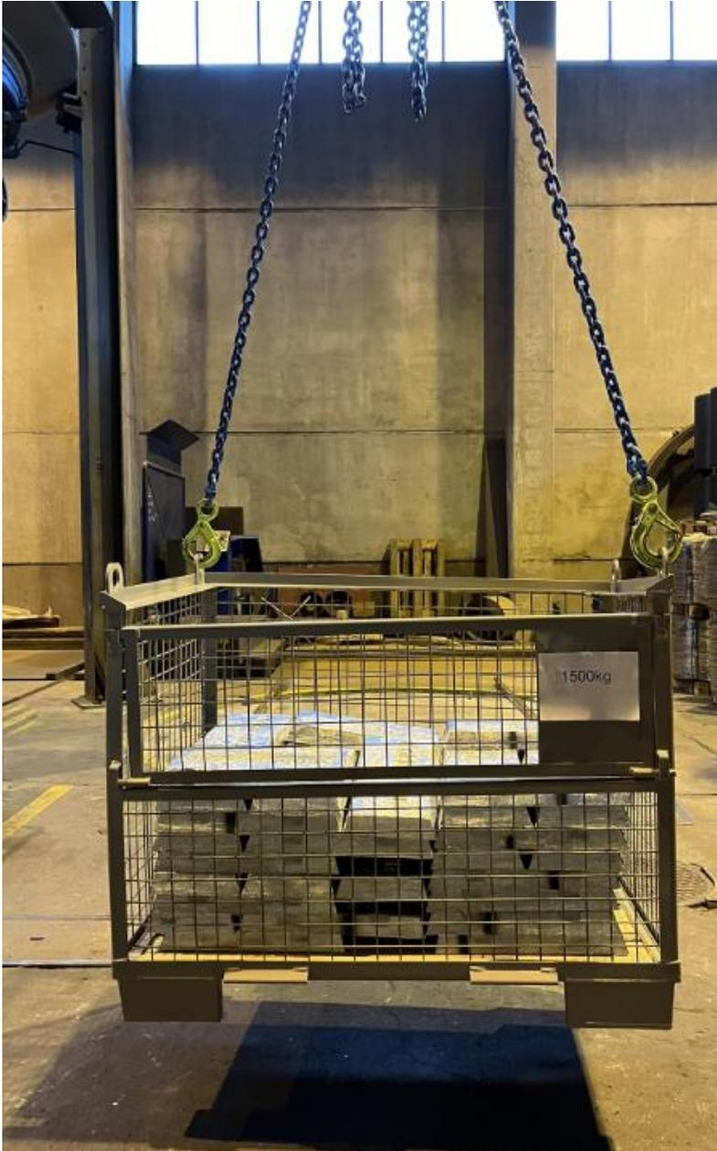
2. Plastic deformation test with 4 out of 4 hooks attached to the Eurobox.
