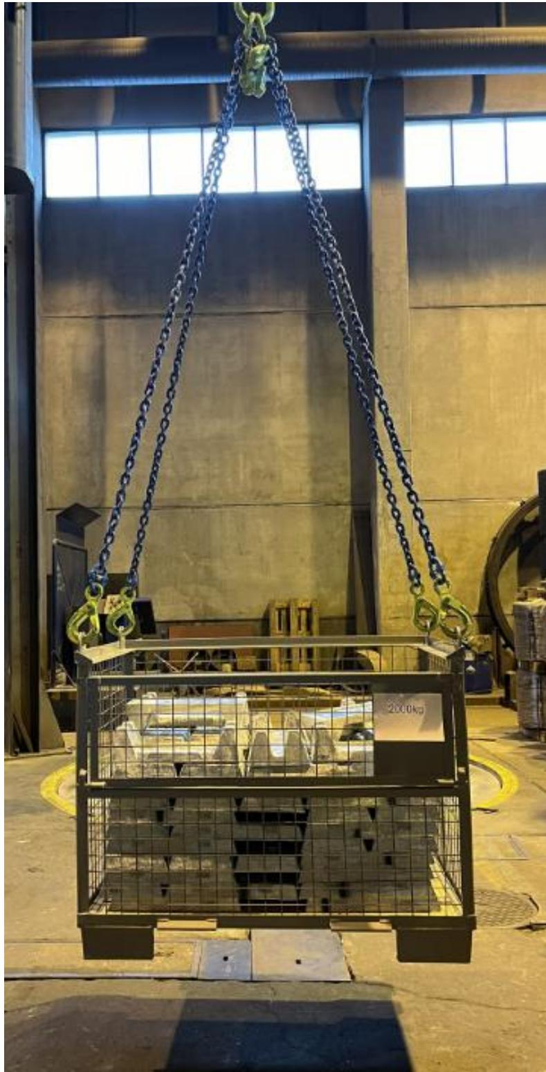
3. Elastic deformation test with 4 out of 4 hooks attached to the Eurobox
